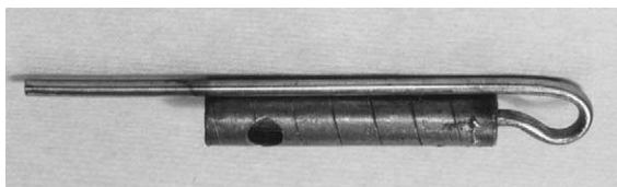
Fig. 3. View of the dip sampler (92 mm length, 12 mm outside diameter).
